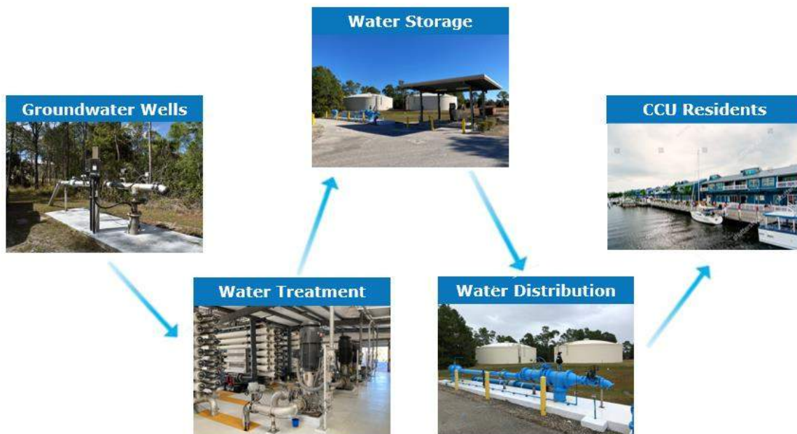
Figure 3-16 Burnt Store Water System Overview
