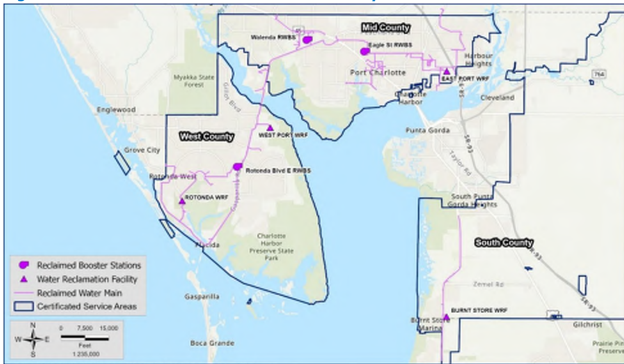
Figure 7-1 CCU Reclaimed Water Distribution Systems
