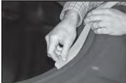
**FIG.2 Apply Gasket**
