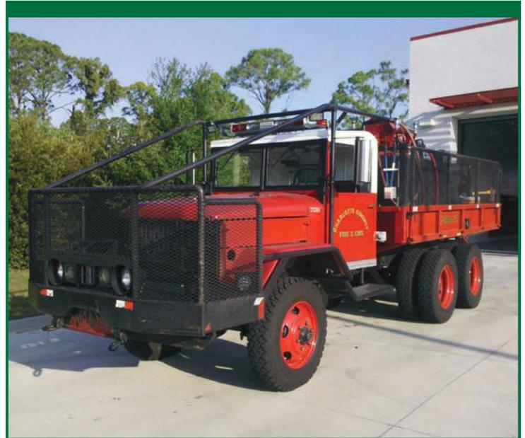
**The Brush 15 Truck and has three drive axles, making it a 6 x 6.**
