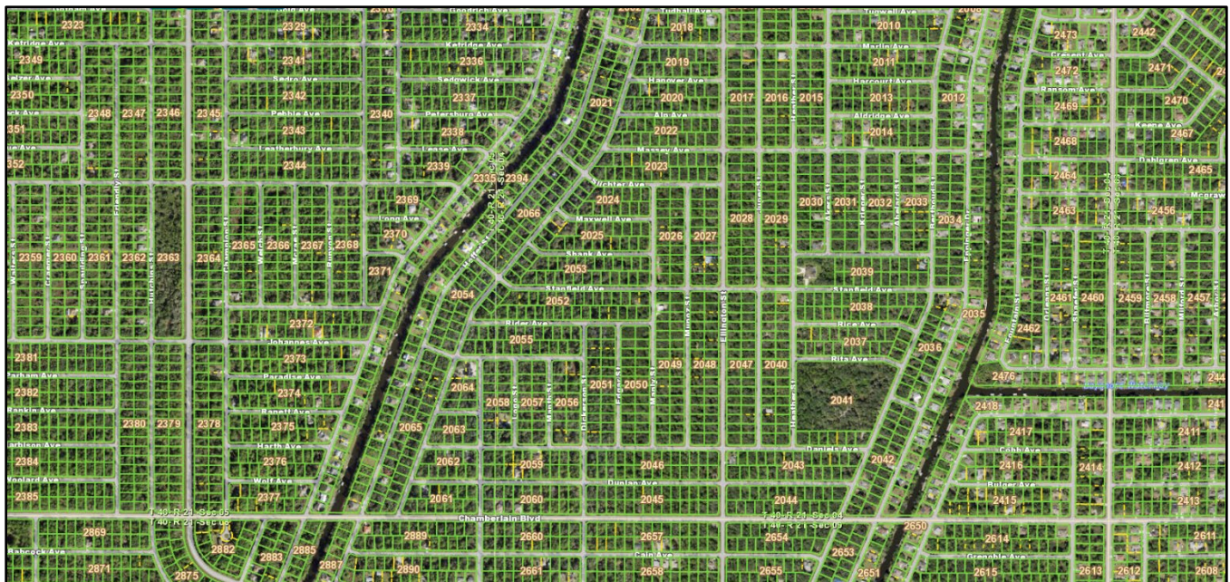
Figure 20. Residential parcels near Port Charlotte. Most of these properties are unimproved (not developed); stormwater volume is expected to increase in this area as these lots are developed.
