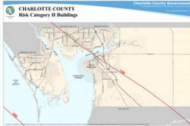
FIGURE 1609A ULTIMATE DESIGN WIND SPEEDS, V_{ult} FOR RISK CATEGORY II BUILDINGS AND OTHER STRUCTURES 2010 FBC
