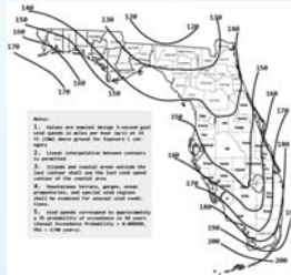
FIGURE 1609B ULTIMATE DESIGN WIND SPEEDS, V_{ult} FOR RISK CATEGORY III AND IV BUILDINGS AND OTHER STRUCTURES 2010 FBC
