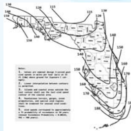
FIGURE 1609A ULTIMATE DESIGN WIND SPEEDS, V_{ult} FOR RISK CATEGORY II BUILDINGS AND OTHER STRUCTURES
