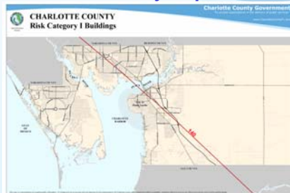
FIGURE 1609C ULTIMATE DESIGN WIND SPEEDS, V_{ult} FOR RISK CATEGORY I BUILDINGS AND OTHER STRUCTURES
